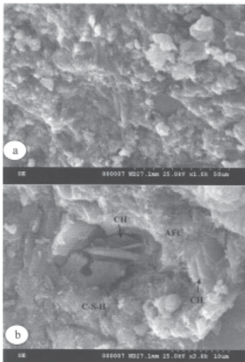
Fig. 11. SEM micrograph of cement paste (E) hydrated 28 days: a) x1000; b) x3000
